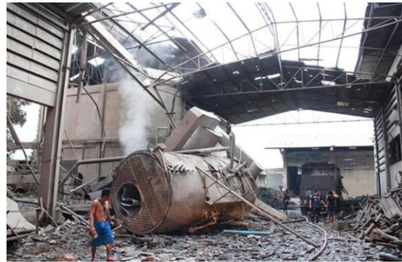
**Fig. 4: Aftermath of a boiler explosion**
