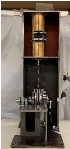
Fig. 1: our new 30 Watt, Uniflow - engine
